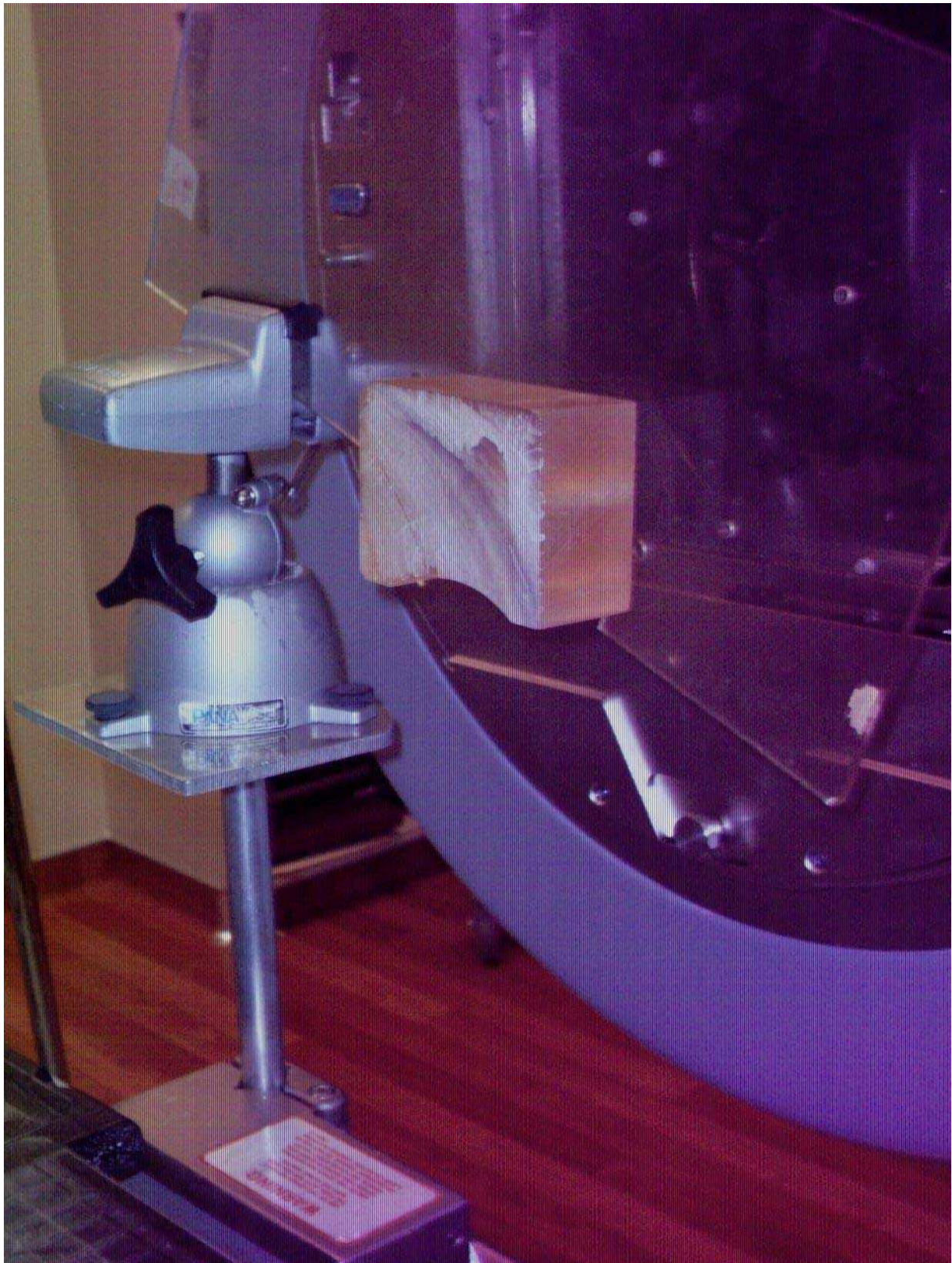
Fig. 2. Acrylic head and neck compensator mounted on post connected to accelerator couch rail arm support.
