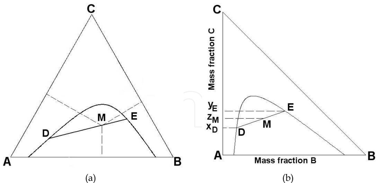
Fig. 8. Liquid-liquid equilibrium; (a) Equilateral triangular coordinates; (b) Rectangular coordinates
