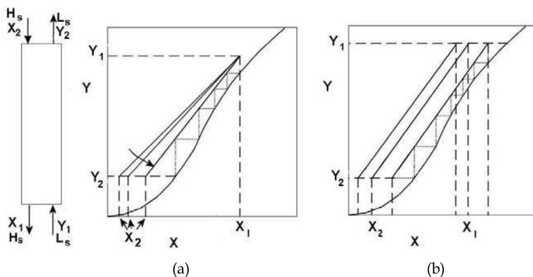
Fig. 16. An absorption-like process; (a) Known three mole ratios ( $X_1$ ,  $Y_1$  and  $Y_2$ ) and five theoretical stages; (b) Known flow rates ( $L_s$ ,  $H_s$ ), two mole ratios ( $Y_1$ ,  $Y_2$ ) and six theoretical stages
