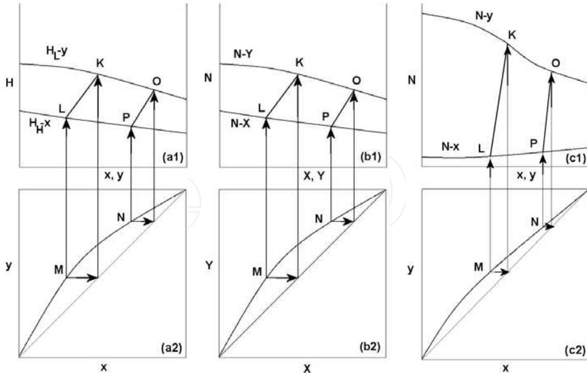
Fig. 17. Useful equilibrium diagrams; (a1, a2)  $Hxy$  diagram useful in distillation operation when using the Ponchon-Savarit method for binary systems; (b1, b2)  $NXY$  diagram used in liquid-liquid extraction; (c1, c2)  $Nxy$  diagram used in leaching operation
