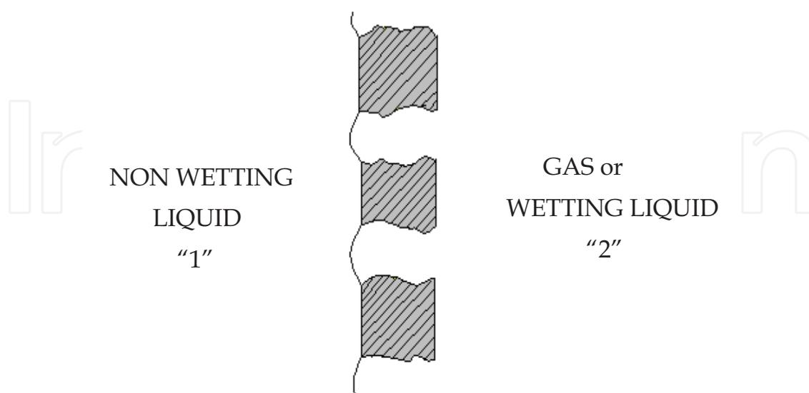
Fig. 1. The membrane contactor concept based on porous hydrophobic membrane in contact with an aqueous (non wetting) liquid at one side and a gas or organic (wetting) liquid at the other side
