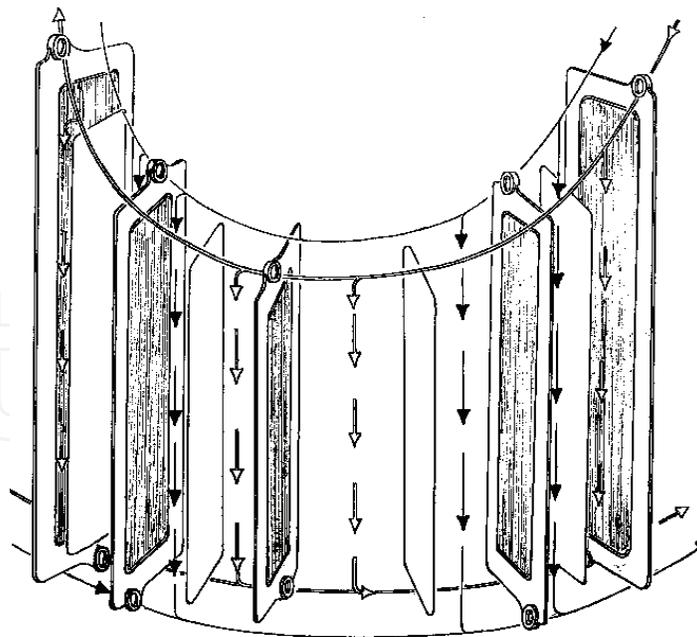
Fig. 2. The concept of plate & frame membrane contactors
