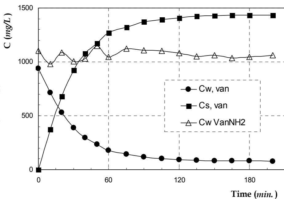
Fig. 13. Vanillin and vanillylamine concentrations vs. time in the extraction with buthyl- acetate. Feed shell side, feed volume 0.5 L, solvent volume 0.3 L, feed flow rate 45 L/h, solvent flow rate 25 L/h, pH 7
