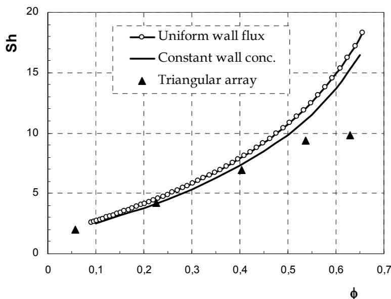
Fig. 11. Asymptotic Sherwood numbers (low  $Gz$ ) for the equivalent annulus model under the conditions of uniform wall flux and constant wall concentration, compared with the data of [Miyatake & Iwashita, 1990] for triangular array
