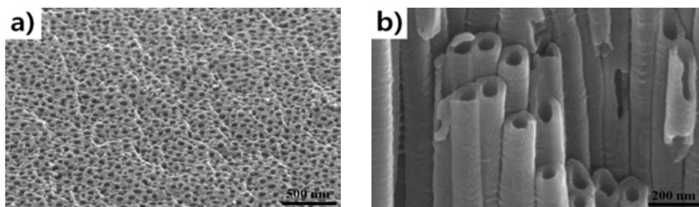
Fig. 9. SEM images of the TiO<sub>2</sub> NT fabricated Ti for 30 min anodizing (a) surface and (b) cross-section. © The Royal Society of Chemistry<sup>[19]</sup>.
