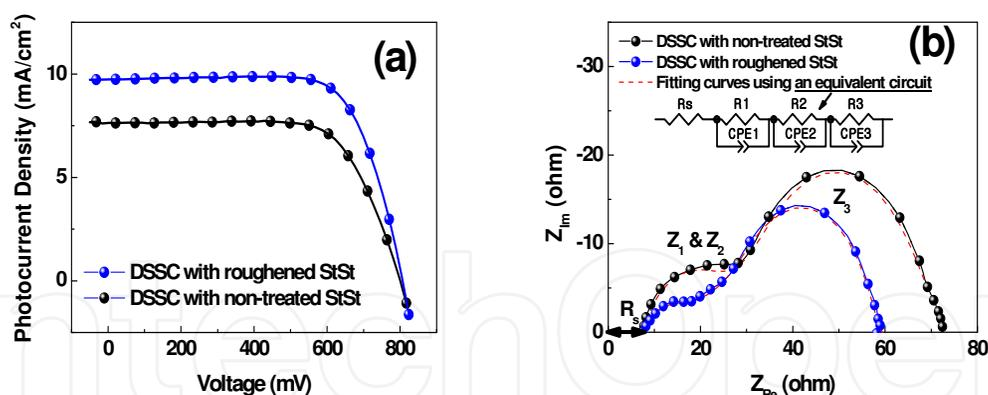
Fig. 3. Under AM 1.5 irradiation ( $100 \text{ mW/cm}^2$ ) with a xenon lamp. (a)  $J$ - $V$  curves of DSSC with nontreated StSt substrates and roughened StSt substrates. (b) Electrochemical impedance spectra measured at the frequency range of  $10^{-1}$ - $10^6$  Hz and fitting curves using an equivalent circuit model including three CPEs. © American Institute of Physics<sup>[17]</sup>.
