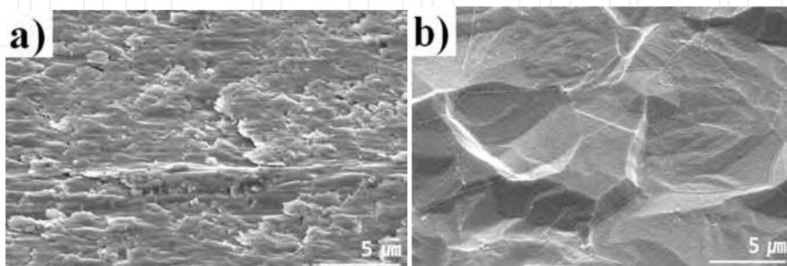
Fig. 4. SEM images of the Ti surface before thermal annealing: (a) non-treated, (b) HF- $\text{HNO}_3$  treated. © WILEY-VCH Verlag GmbH & Co. KGaA, Weinheim<sup>[18]</sup>.
