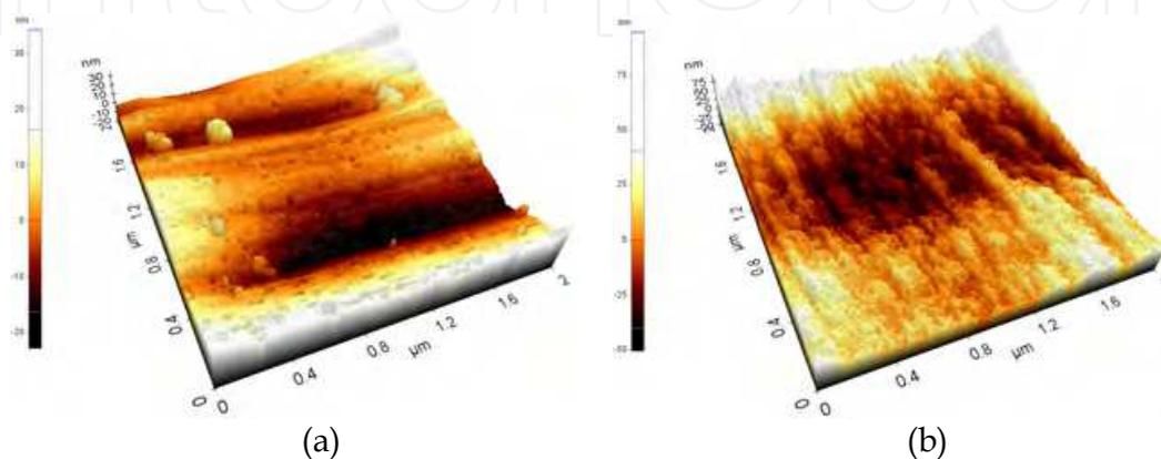
Fig. 2. AFM images of StSt surface (a) before and (b) after roughening process. © American Institute of Physics<sup>[17]</sup>.
