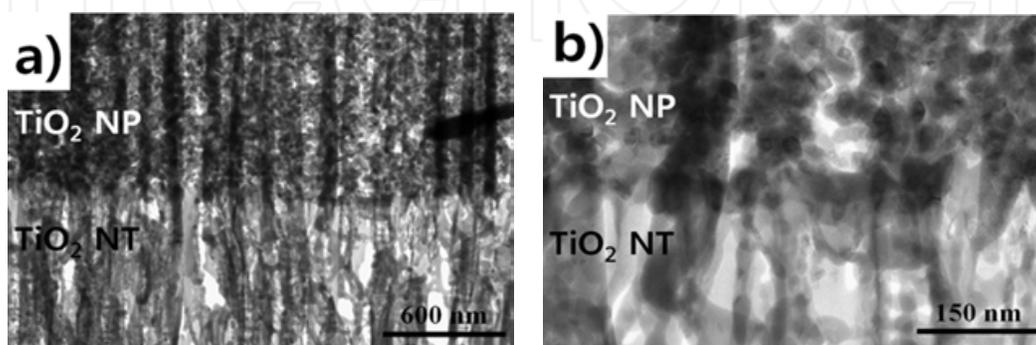
Fig. 10. Cross-sectional TEM images of (a) interface between TiO<sub>2</sub> NP and TiO<sub>2</sub> NT (b) magnified view of (a). © The Royal Society of Chemistry<sup>[19]</sup>.
