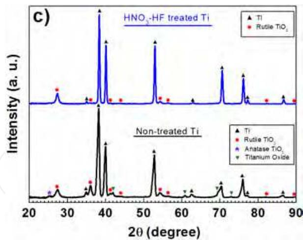
Fig. 7. By use of a  $2\theta$  scan method, XRD patterns of non-treated and  $\text{HNO}_3$ -HF-treated Ti substrates after thermal annealing at  $550^\circ\text{C}$  for 30 min. © WILEY-VCH Verlag GmbH & Co. KGaA, Weinheim<sup>[18]</sup>.
