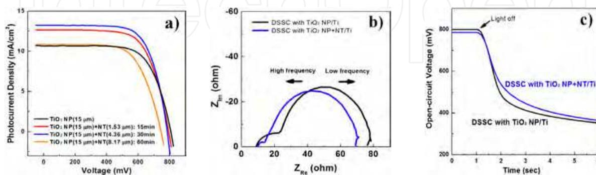
Fig. 11. (a)  $J$ - $V$  characteristics of the DSSC with TiO<sub>2</sub> NP/Ti and TiO<sub>2</sub> NP + NT/Ti. (b) Electrochemical impedance spectra in frequencies ranging from 10<sup>-1</sup> to 10<sup>6</sup> Hz. (c) Open-circuit voltage decay measurement. © The Royal Society of Chemistry<sup>[19]</sup>.
