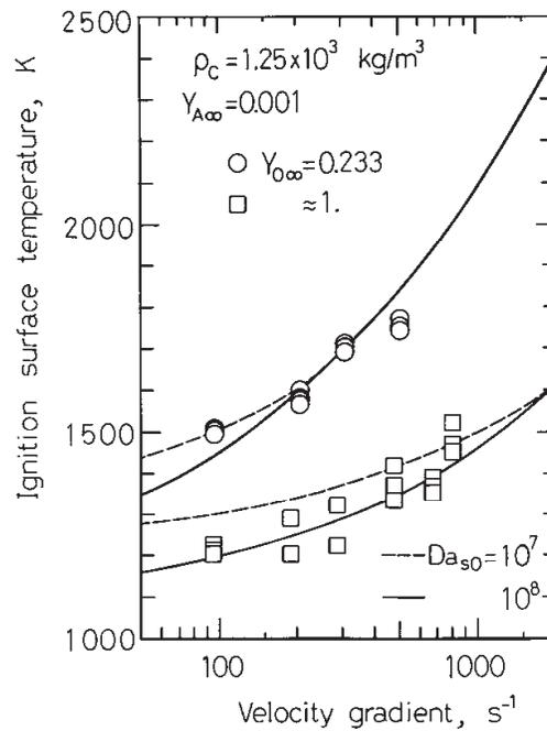
Fig. 4. Surface temperature at the establishment of CO-flame, as a function of the stagnation velocity gradient, with the O<sub>2</sub> mass-fraction in the freestream and the surface Damköhler number for the C-O<sub>2</sub> reaction taken as parameters. Data points are experimental (Makino, et al., 1996) with the test specimen of 10 mm in diameter and  $1.25 \times 10^3 \text{ kg/m}^3$  in graphite density; curves are calculated from theory (Makino & Law, 1990).
