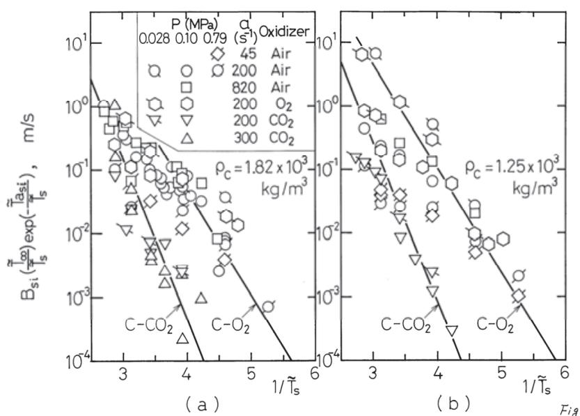
Fig. 6. Arrhenius plot of the surface C-O<sub>2</sub> and C-CO<sub>2</sub> reactions (Makino, et al., 1994), obtained from the experimental results of the combustion rate in oxidizer-flow of various velocity gradients; (a) for the test specimen of  $1.82 \times 10^3$  kg/m<sup>3</sup> in graphite density; (b) for the test specimen of  $1.25 \times 10^3$  kg/m<sup>3</sup> in graphite density.
