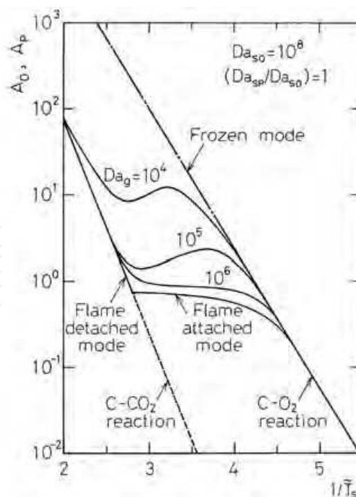
Fig. 5. Arrhenius plot of the reduced surface Damköhler number with the gas-phase Damköhler number taken as a parameter;  $Da_{s,O} = Da_{s,P} = 10^8$ ;  $Da_{s,P}/Da_{s,O} = 1$ ;  $Y_{O,\infty} = 0.233$ ;  $Y_{P,\infty} = 0$  (Makino, et al., 1994).
