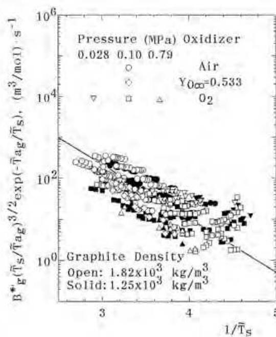
Fig. 7. Arrhenius plot of the global gas-phase reaction (Makino, et al., 1994), obtained from the experimental results of the ignition surface-temperature for the test specimens ( $1.82 \times 10^3$  kg/m<sup>3</sup> and  $1.25 \times 10^3$  kg/m<sup>3</sup> in graphite density) in oxidizer-flow at various pressures, O<sub>2</sub>, and H<sub>2</sub>O concentrations .
