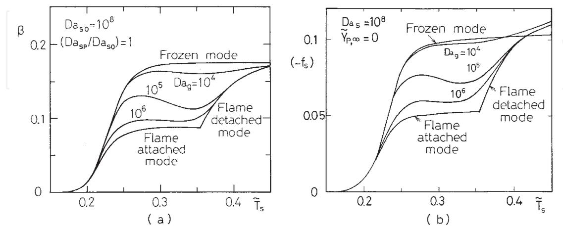
Fig. 1. Combustion behavior as a function of the surface temperature with the gas-phase Damköhler number taken as a parameter;  $Da_{s,O}=Da_{s,P}=10^8$  and  $Y_{P,\infty}=0$  (Makino, 1990). (a) Transfer number. (b) Nondimensional combustion rate.
