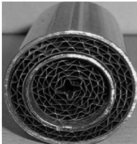
Fig. 11. Metallic-made monolithic reactor (Source: Mei et al., 2007)
