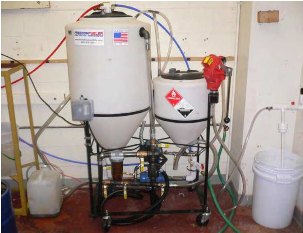
Fig. 3. Biodiesel Processor with a capacity of 40 gallons/day
