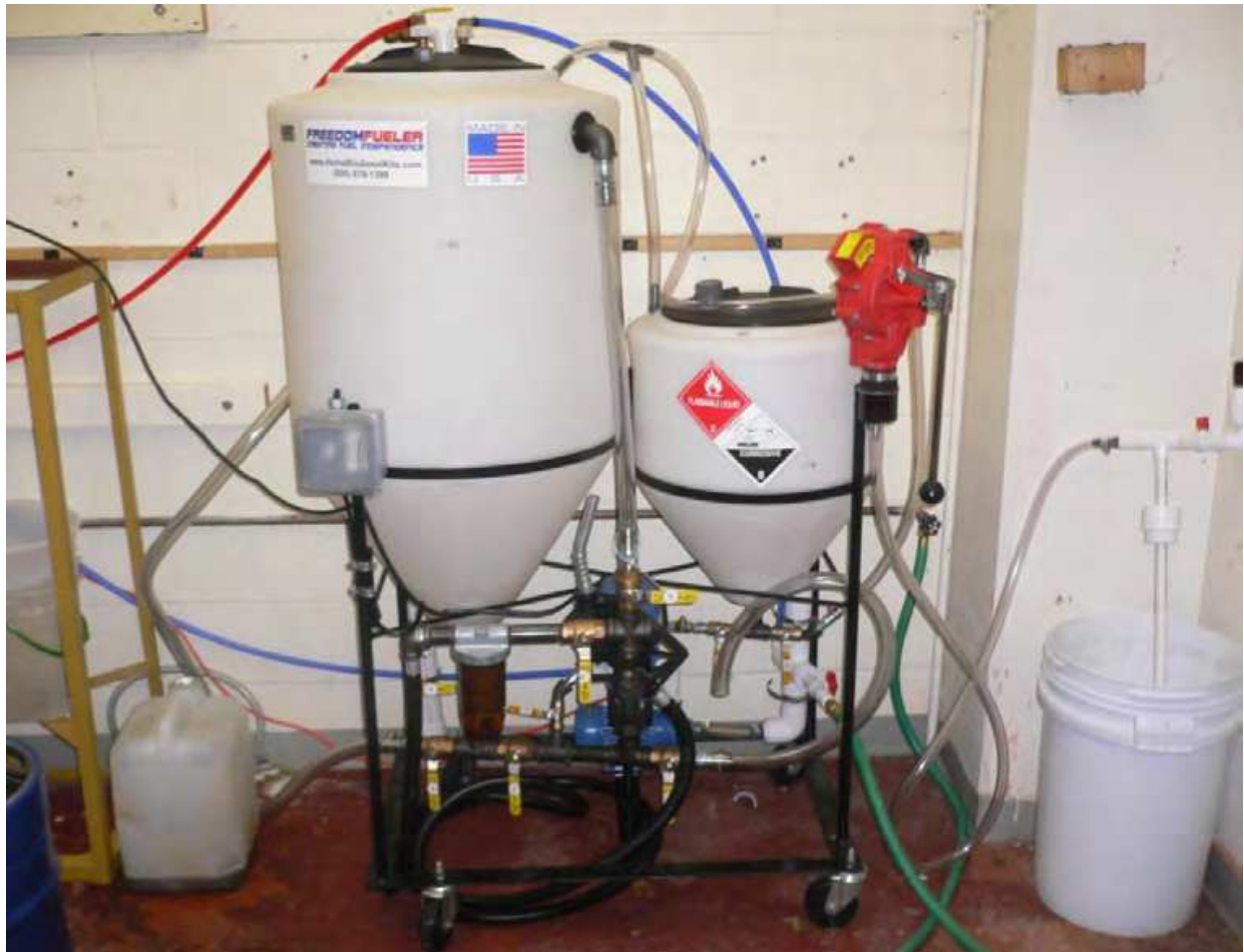
Fig. 3. Biodiesel Processor with a capacity of 40 gallons/day
