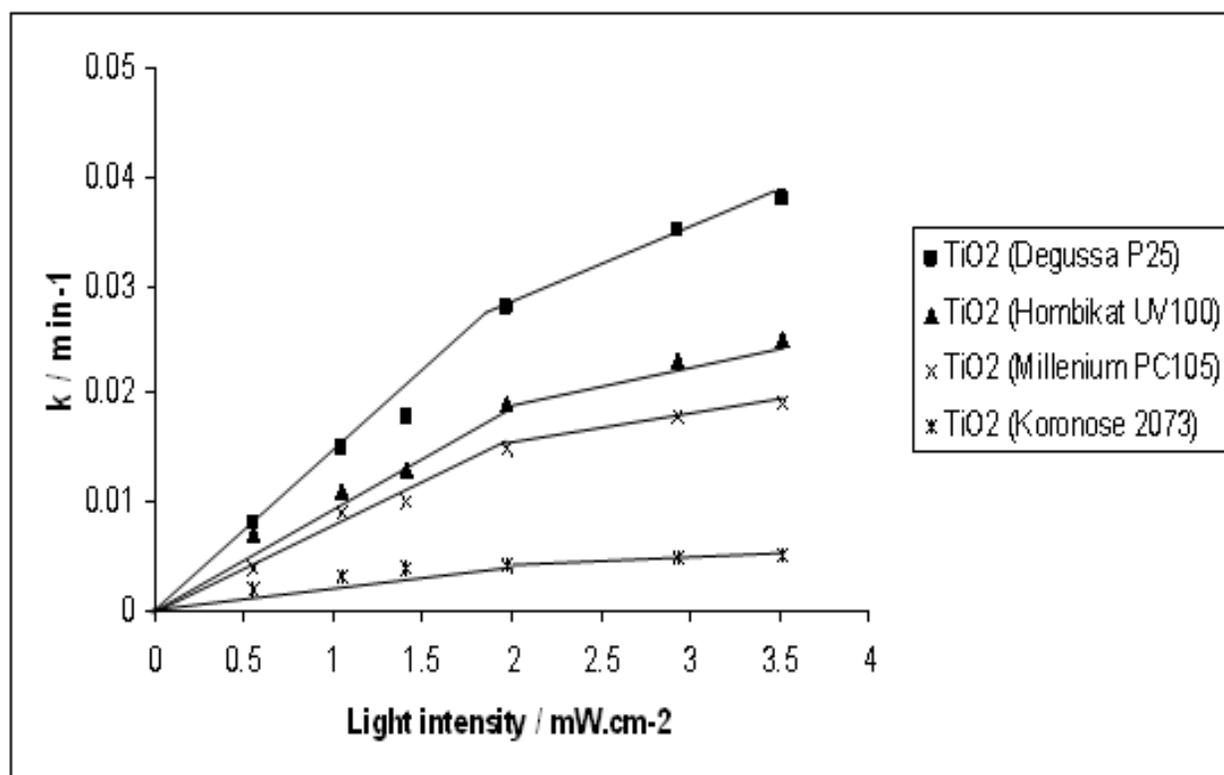
Fig. 12. Effect of initial light intensity on rate constant of photocatalytic decolorization of Bismarck brown R using different types of TiO<sub>2</sub>
