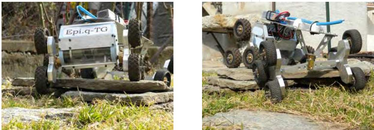
Fig. 17. Epi.q-2 traversing an obstacle, on uneven ground
