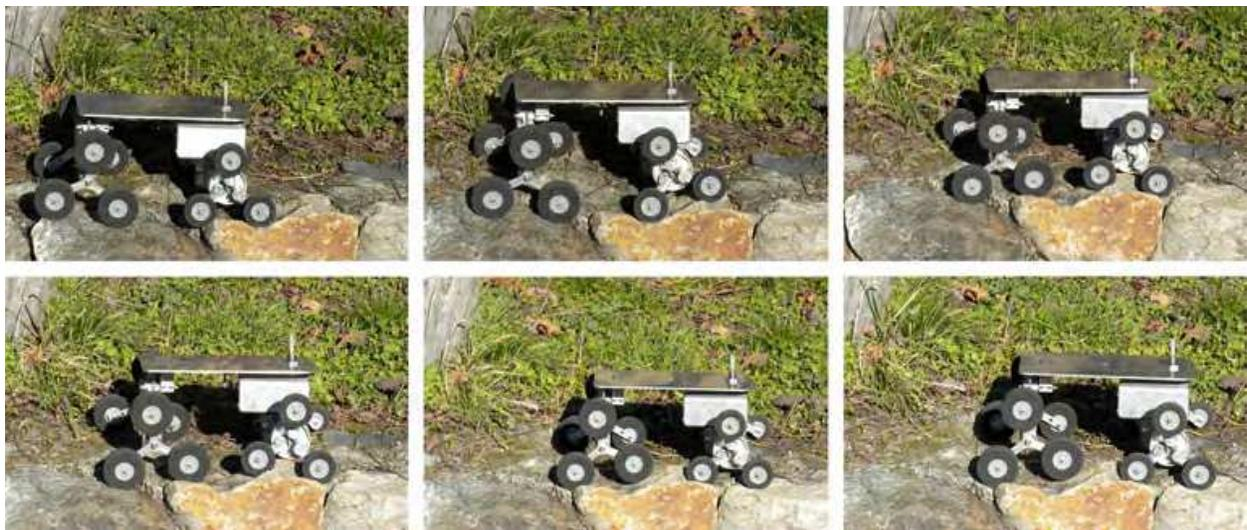
Fig. 12. Epi.q-1 in advancing mode, on uneven ground
