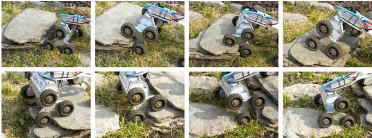
Fig. 13. Epi.q-2 negotiating an obstacle
