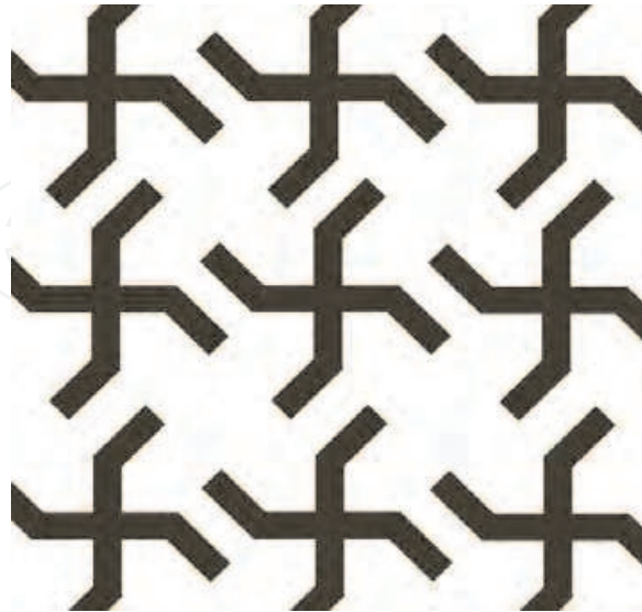
Fig. 4. Planar chiral structure made by arrays of gammadions arranged in two-dimensional square gratings (Papakostas et al., 2003).
