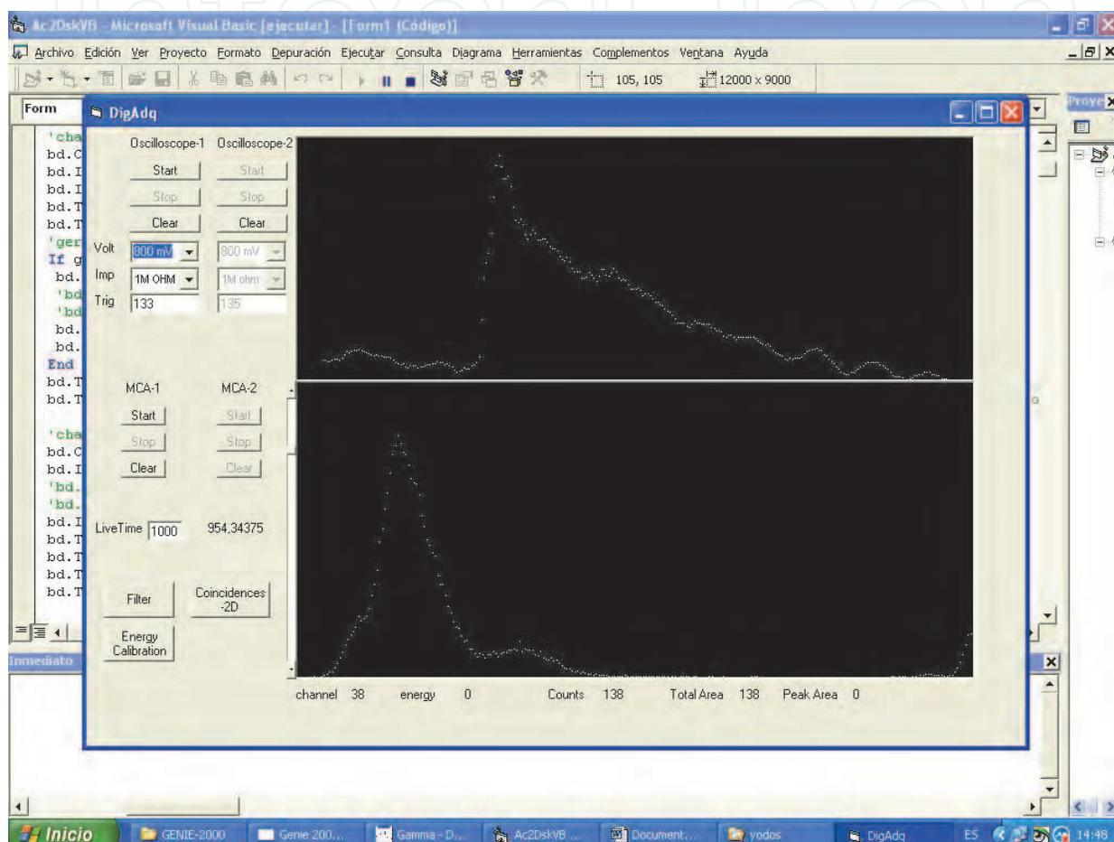
Fig. 5. Alpha spectrum of a radium sample in an aqueous medium using alpha/beta Ultima-Gold scintillator. The large peak corresponds to Ra-226 (4.7 MeV) and its descendents Po-210 (5.3 MeV), Rn-222 (5.49 MeV), and Pb-218 (6.0 MeV). They interfered and formed a unique peak. The small peak to the right is Po-214 (7.69 MeV). The upper part of the figure shows the shape of the electronic pulse at the preamplifier output. Each point of the pulse graph corresponds to 20 nsec.
