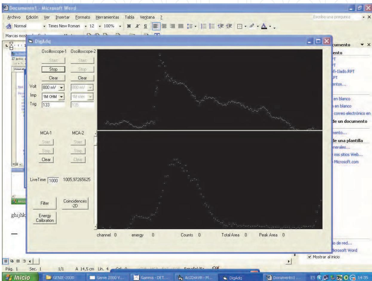
Fig. 4. Alpha spectrum of a uranium sample obtained by liquid-liquid extraction with organic solvents. The energy resolution was about 10% (0.5 MeV) and the peaks of U-238 (4.2 MeV) and U-234 (4.7 MeV) interfered. The upper part of the figure shows the shape of the electronic pulse at the preamplifier output. Each point of the pulse graph corresponds to 20 nsec.
