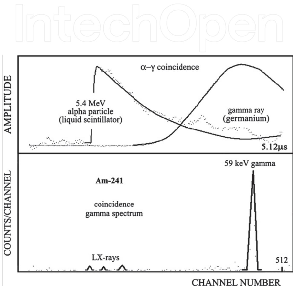
Fig. 6. Am-241 alpha/gamma coincident pulses (above) and coincident gamma spectrum (below) using liquid scintillation and a low energy germanium detector.
