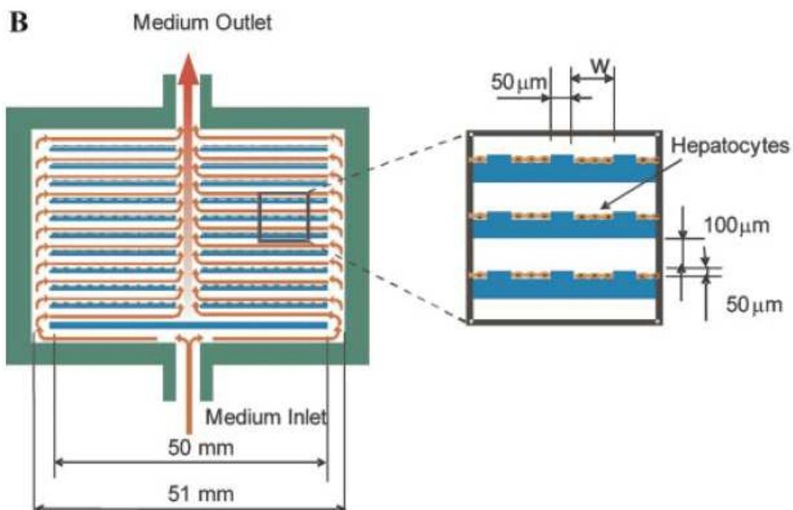
Fig. 5. **Schematic of a radial flow Bioartificial Liver Device.** Red arrows show the direction of medium flow and in blue is the location of the seeded hepatocytes. The design includes patterned microgrooves to decrease shear stress on the seeded hepatocytes. (Figure taken from [67], Figure 1)
