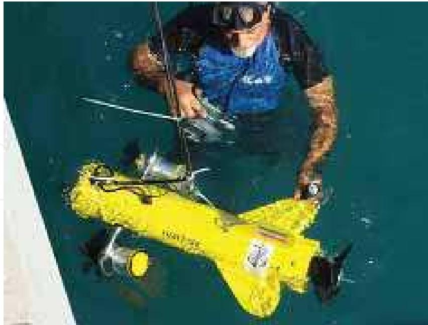
Fig. 4. The proposed ROV and incorporated diagnostic arm for inspection and NDT of a quay wall in Shahid-Rajaei harbor
