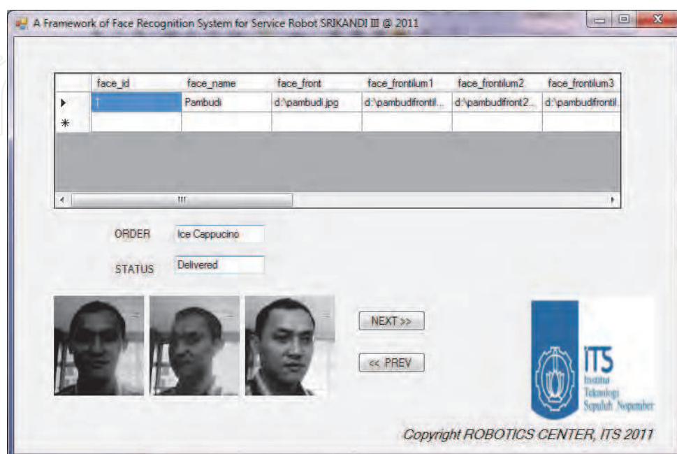
Fig. 3. We have proposed face databases using 1 table, 3 images used for each person (frontal, left and right poses).
