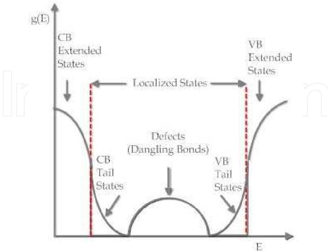
Fig. 4. A schematic representation of the electronic density of states,  $g(E)$ , of a-Si:H. VB indicates the valence band and CB the conduction band. The dashed, red, vertical lines show the mobility edges, which are defined as the energy level separating extended (non-localized) states from localized states.
