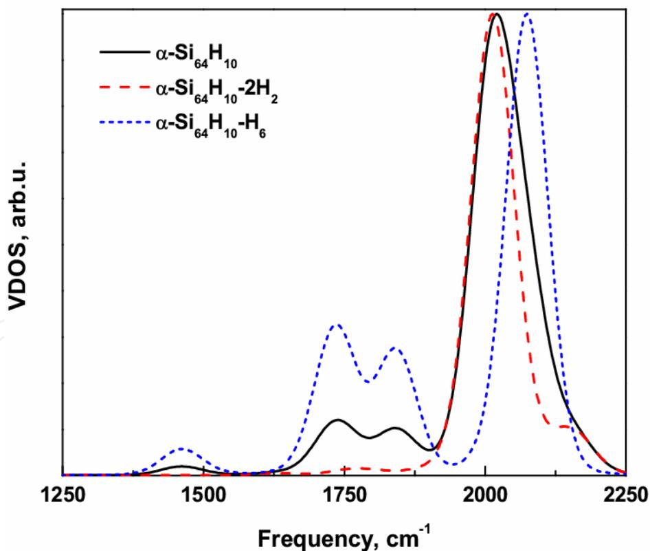
Fig. 10. Hydrogen stretch vibrations for a-Si<sub>64</sub>-H<sub>10</sub> system at high frequency (Kupchak *et al.*, 2008). The solid black line shows all H-associated stretching vibrations, including dihydride modes (blue, short dash) and monohydride modes (red, long dash). Note the very close agreement with data by Lucovsky *et al.* (1989).
