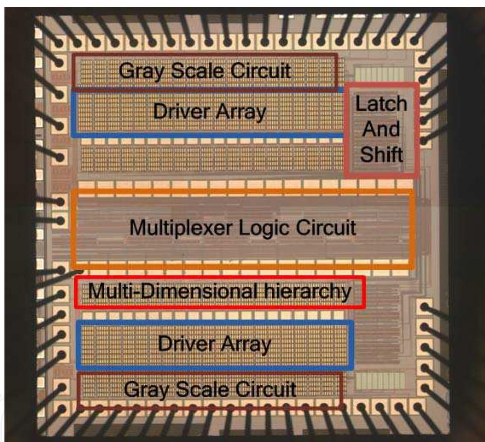
Fig. 14. Photograph of fabricated control IC chip.
