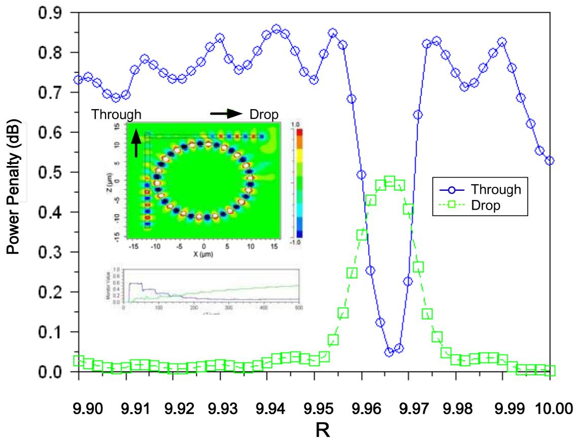
Fig. 2. Transmittance for the radius of micro ring.
