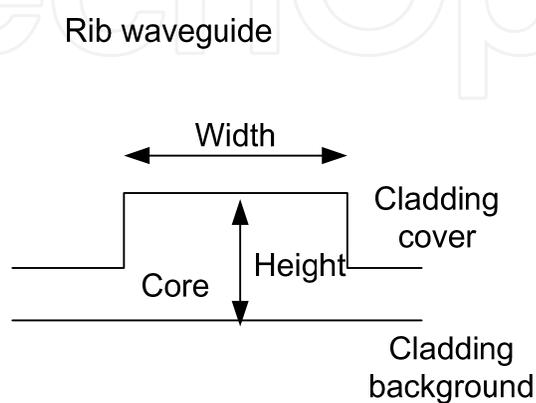
Fig. 3. Schematic cross section of a rib waveguide.
