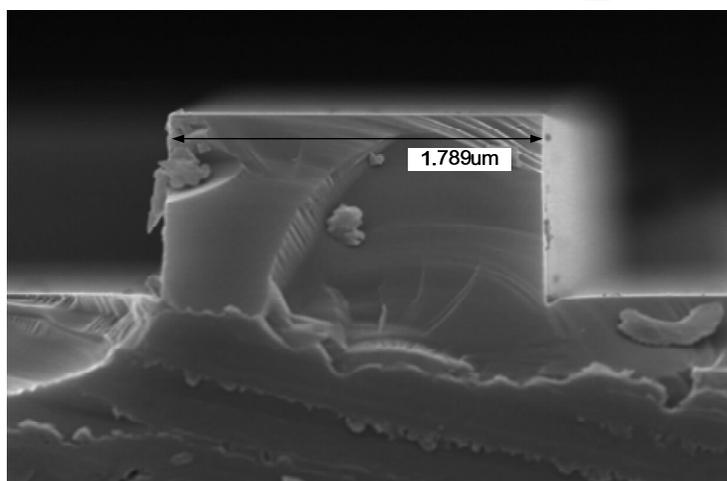
Fig. 5. SEM image of the waveguide cross section.
