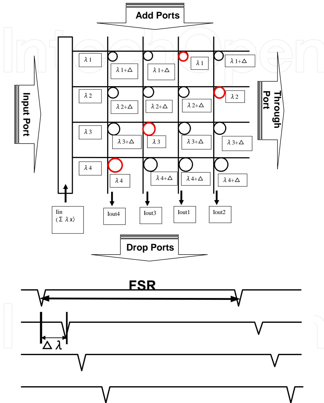
Fig. 1. Schematic of a four-channel PLC.
