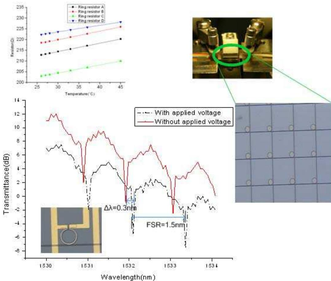
Fig. 16. Wavelength shift of transmission spectrum in coupled-ring-resonator.
