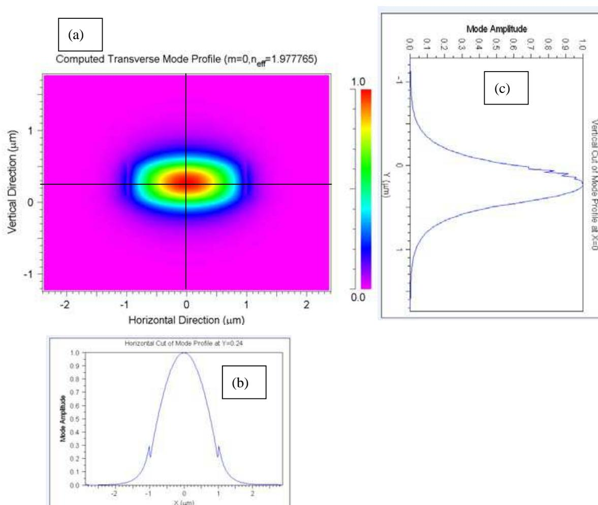
Fig. 4. Simulated fundamental mode profile from BPM-based calculations.
