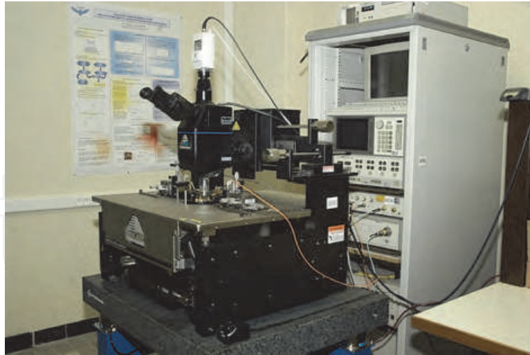
Fig. 19. RF probe station connected with a vector network analyzer
