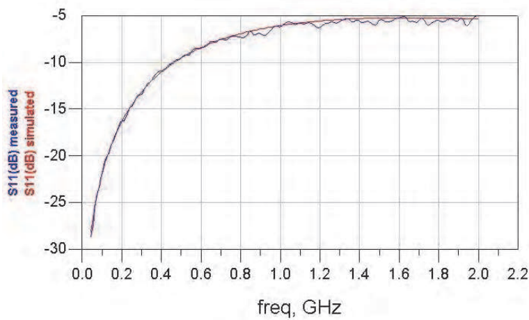
Fig. 26. Measured and simulated S_{11} DBR with 10\mu m ring contact
