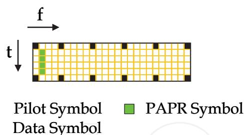
Fig. 5. Structure of a data tile in the RL.
