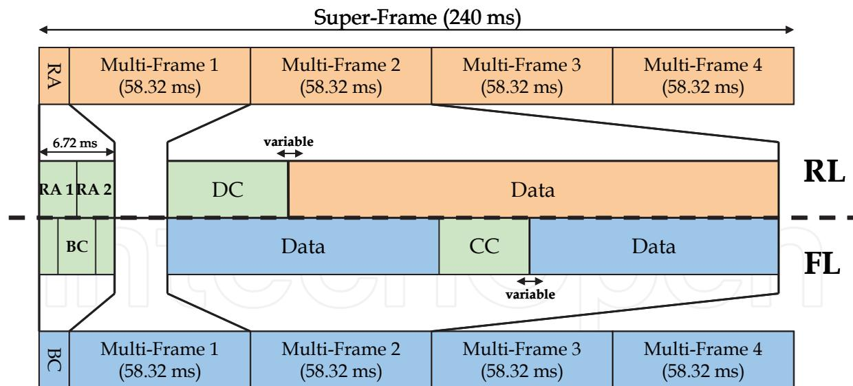
Fig. 11. Super-Frame Structure.
