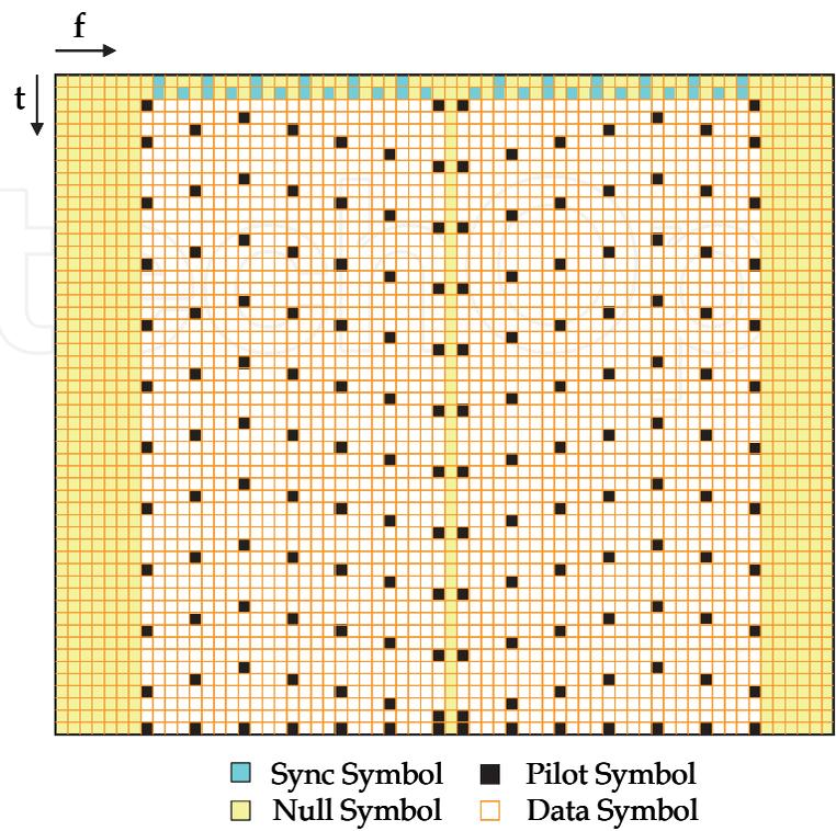
Fig. 3. Structure of a FL Data/CC frame.
