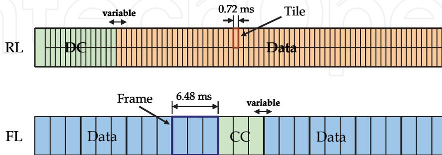
Fig. 10. Multi-Frame structures.
