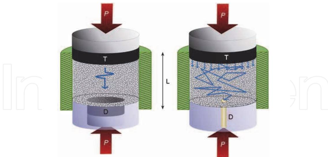
Fig. 1. Multiple scattering of elastic waves in a confined granular packing under stress  $P$ . "T" and "D" correspond to a large source transducer and a small detector, respectively. (Reprinted from Jia et al., Chinese Sci. Bull. 54, 4327 (2009))
