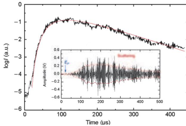
Fig. 3. Averaged time-dependent transmitted intensity  $I(t)$  of the scattered waves traveling across a granular sample of height  $L = 11$  mm. Solid line corresponds to the theoretical solution (58) with the fitting parameters  $D = 0.13 \text{ m}^2/\text{s}$  and  $Q^{-1} = 0.005$ . Inset: Transmitted ultrasonic signal at a given configuration. Dashed lines correspond to the average amplitude profile. (Reprinted from Jia et al., Chinese Sci. Bull. 54, 4327 (2009))
