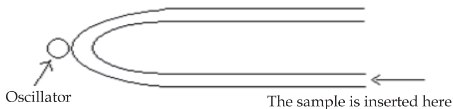
Fig. 7. U-shaped tube of digital density meter.
