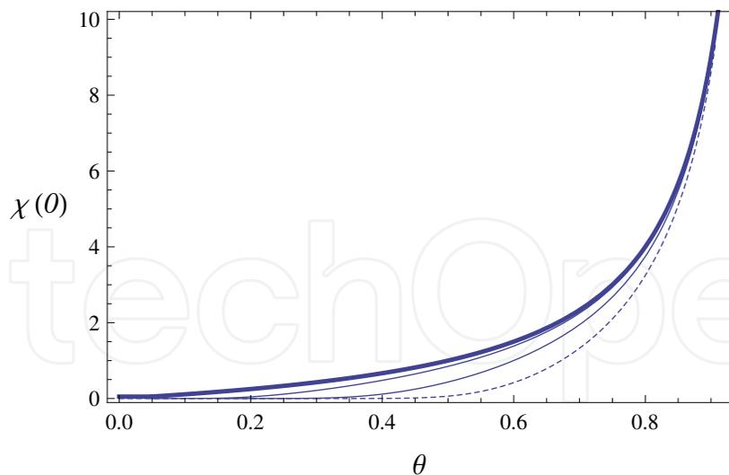
Fig. 4. The maximal efficiency  $\chi(0) = \chi(W = 0)$  given by (??) versus  $\theta = T_c/T_h$  for  $n = 2$  (top normal curve),  $n = 101$  (bottom normal curve), and  $n = 10^5$  (dotted curve). Thick curve: the efficiency  $\theta/(1 - \theta)$ .
