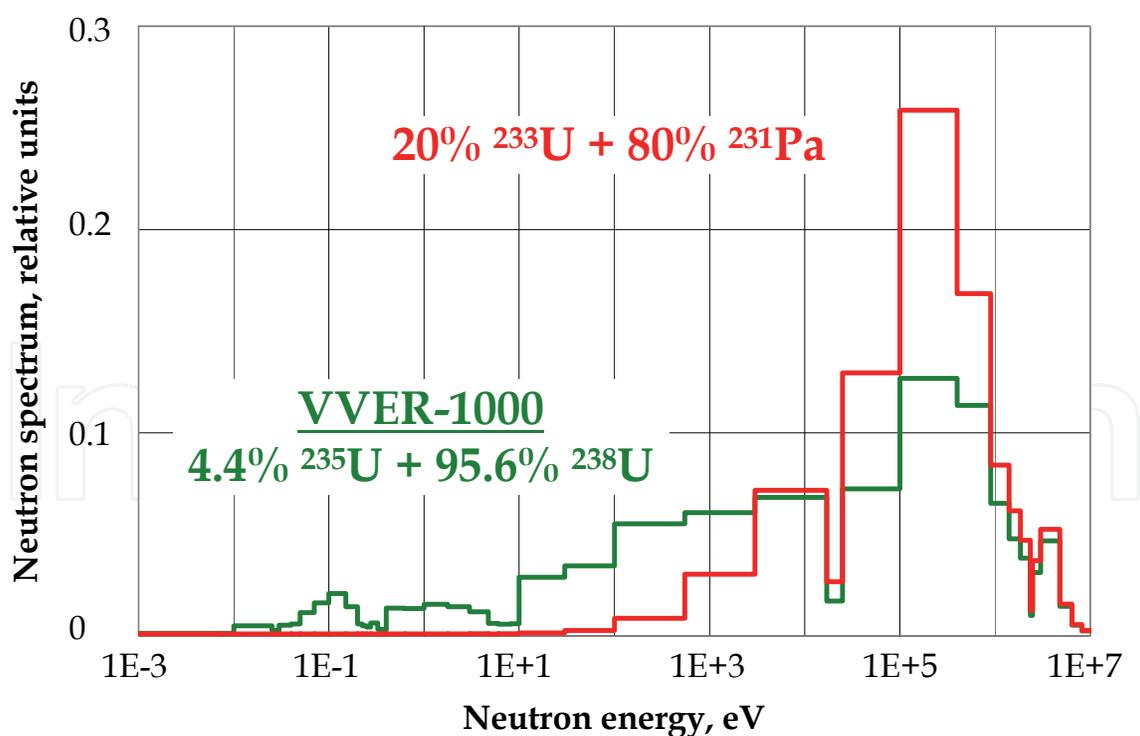
Fig. 2.  $^{231}\text{Pa}$  effect on energy spectrum of neutrons
