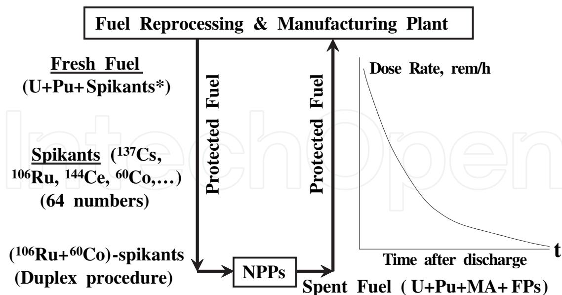
Fig. 12. Closed (U-Pu)-fule cycle protected (ORNL, USA)\*
