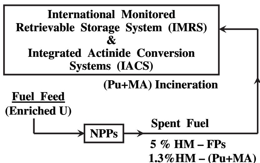
Fig. 13. Open fuel cycle protected (LANL, USA)
