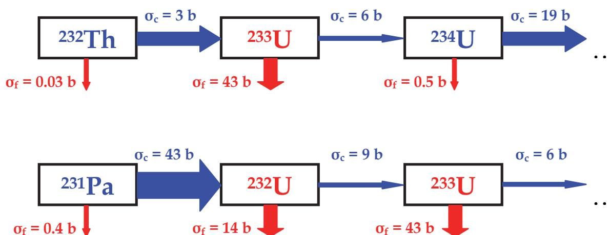
Fig. 6. Chains of isotopic transformations ( $^{232}\text{Th} \rightarrow ^{233}\text{U} \rightarrow ^{234}\text{U} \rightarrow \dots$ ) and ( $^{231}\text{Pa} \rightarrow ^{232}\text{U} \rightarrow ^{233}\text{U} \rightarrow \dots$ ) (neutron spectrum of VVER-1000)
