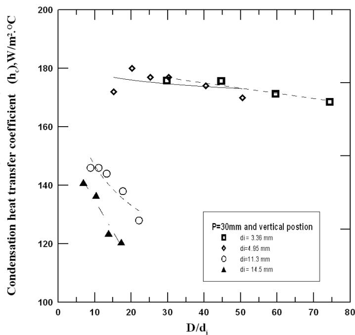
Fig. 11. Condensation heat transfer coefficient versus  $D/d_i$  ratio.
