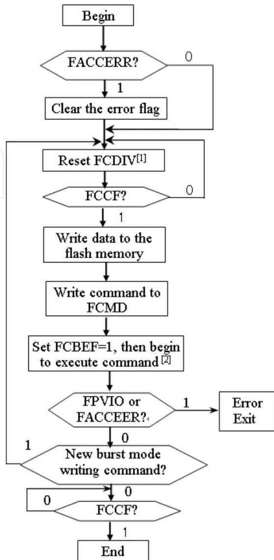
Fig. 3. AW60 Flash burst mode programming flowchart
