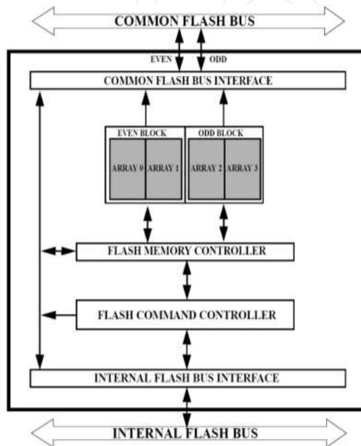
Fig. 10. CFM Block Diagram
