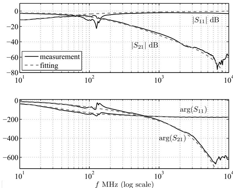
Fig. 12. Selection of the scattering responses of the power rail structure carried out between the first and the last pair of  $VDDQ$ - $VSSQ$  pads, for the example test-case. Solid line: on-chip measurements; dashed line: responses by means of the simplified equivalent of Fig. 3c.
