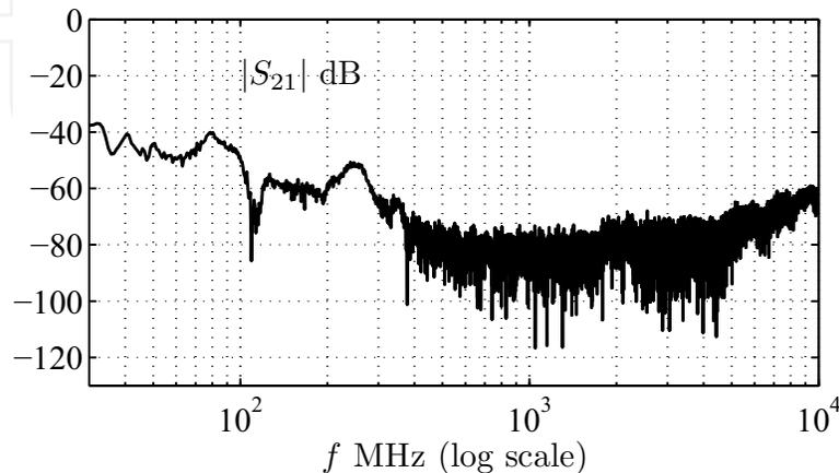
Fig. 2. On-chip measurement of the S21 scattering parameter carried out between two heterogeneous pairs of VDD $n$ -VSS $n$  and VDDQ $n$ -VSSQ $n$  supply pads. The measurement highlights the low coupling between the core and the buffer power delivery networks for the example test chip considered in the study.
