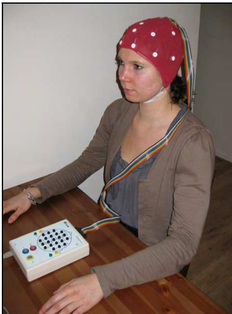
Fig. 2. An example of the set up of a 19-channel EEG assessment using the Mitsar EEG 201 System.
