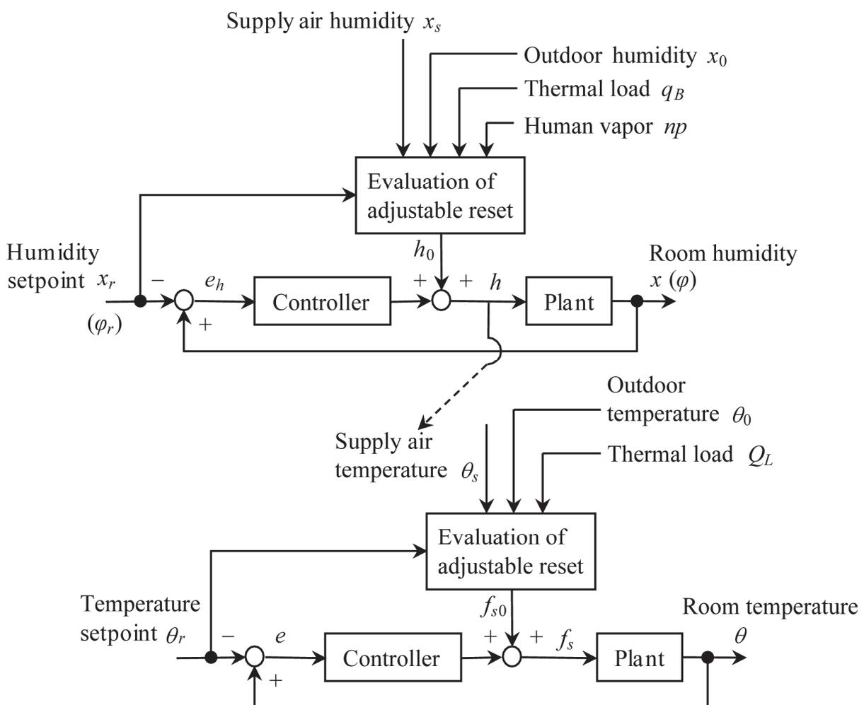
Fig. 3. Overall of the temperature-humidity control system.
