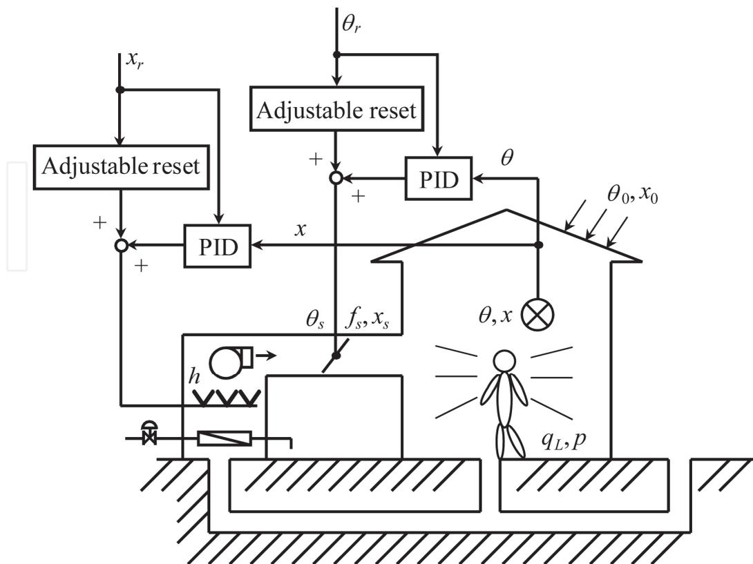
Fig. 1. Overall structure of a single-zone cooling system.
