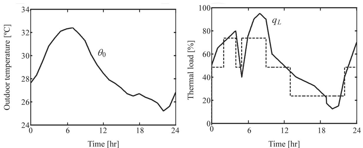
Fig. 4. Outdoor temperature and thermal loads profiles.
