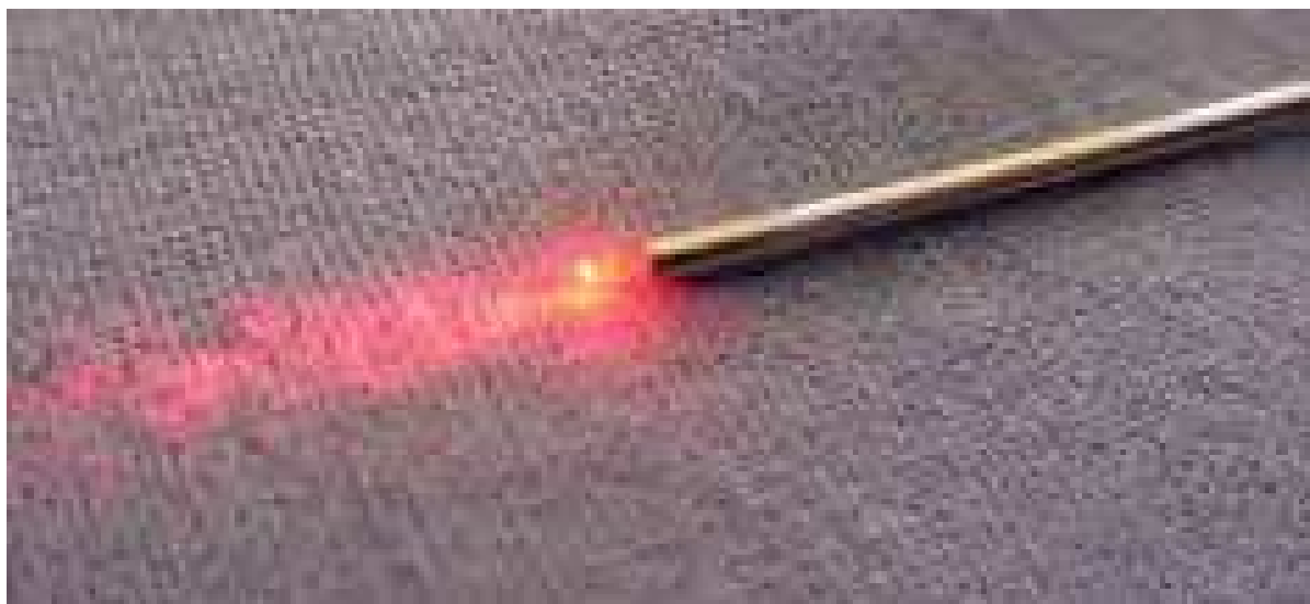
Fig. 4. One-millimeter cannula containing fiber optic extended approximately 2mm from the distal end and emitting laser energy.
