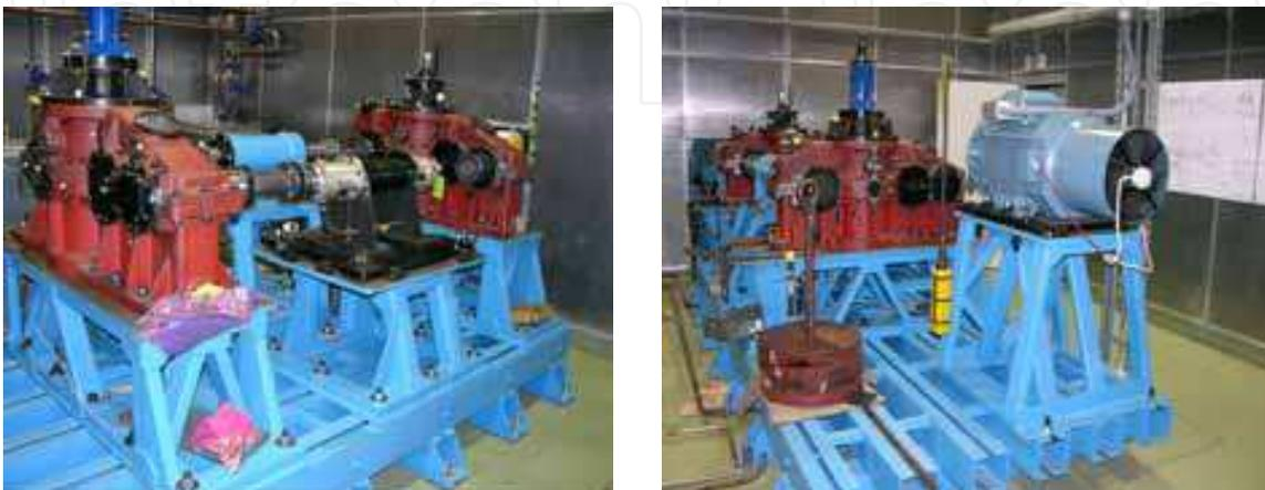
Fig. 3. Gear fatigue test rig overall view
