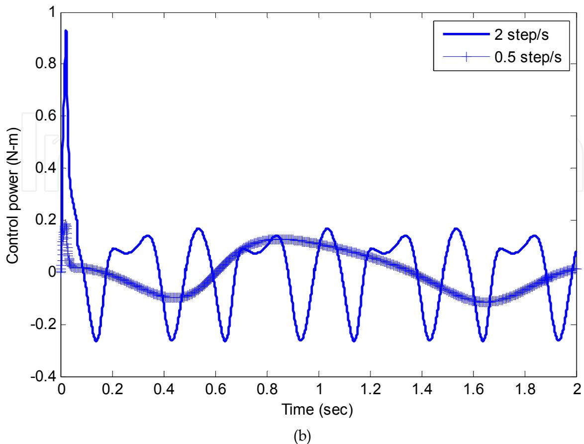
Fig. 10. Control power for DTC and DFC methods.
