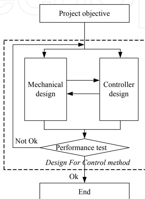
Fig. 8. Integrated design of mechatronic system using DFC.
