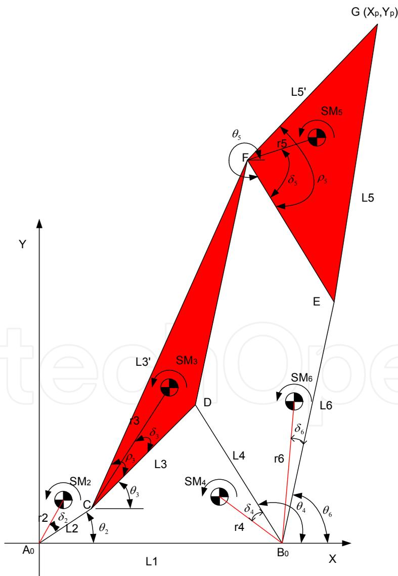
Fig. 7. Dynamic model of linkage for Leg system.
