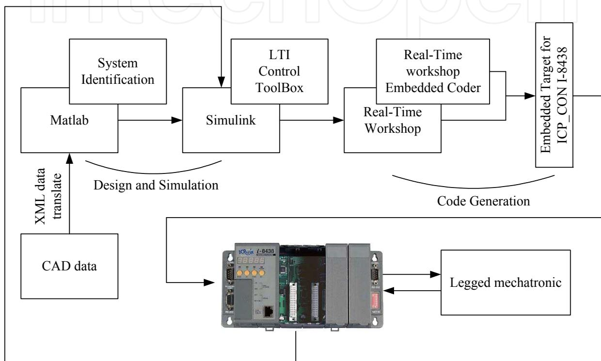
Fig. 4. Legged mechatronic system design flow chart.
