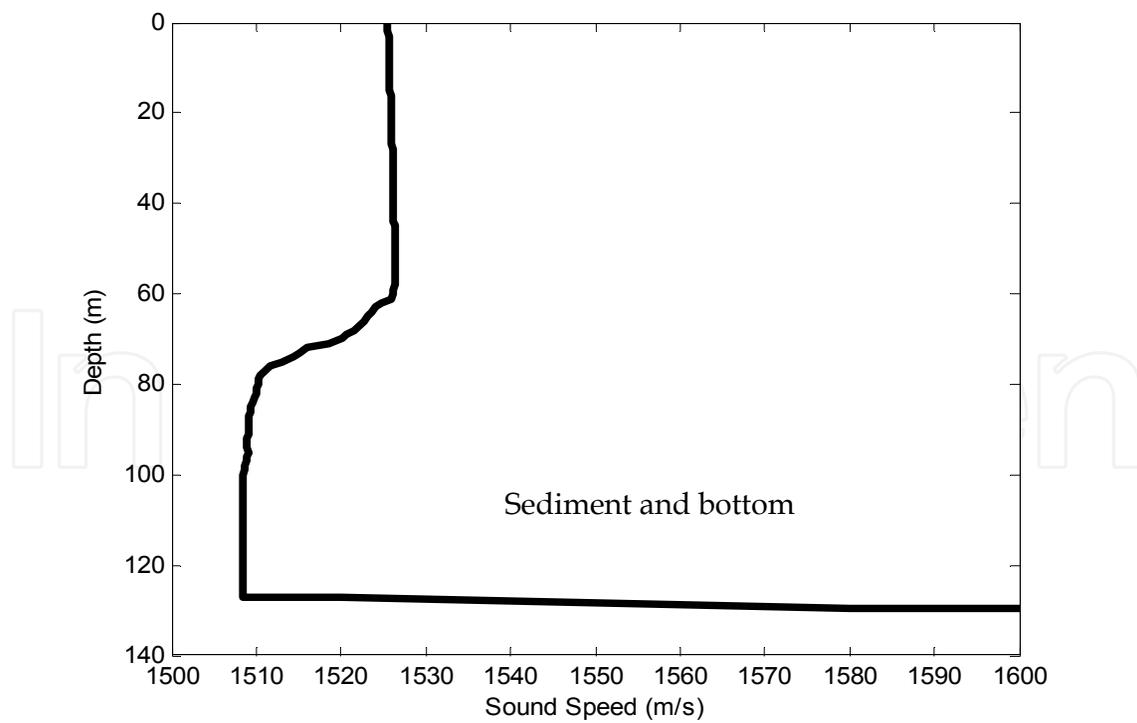
Fig. 10. Measured Sound Speed Profile of SCALANTC 1993 North Elba experiment.
