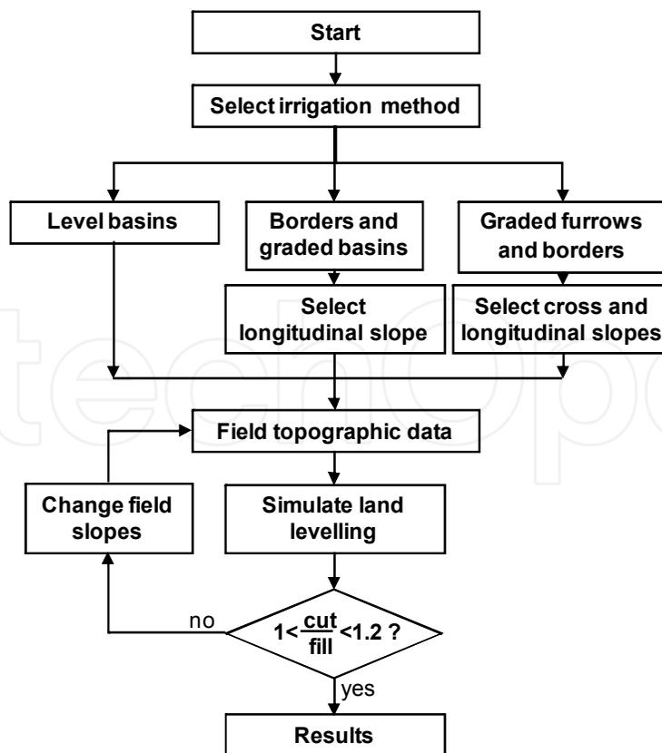
Fig. 5. Flowchart of the application of the land leveling simulation tool.
