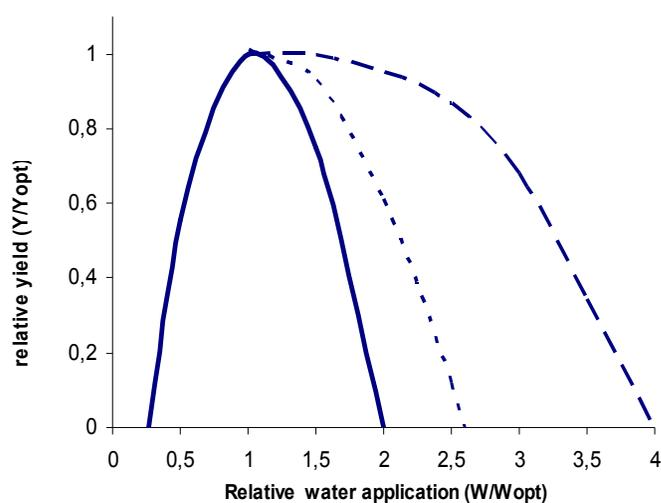
Fig. 6. Irrigation water-yield functions. Examples of quadratic equations with different descending branches for a crop susceptible to excess water in a poorly drained soil (—), for a susceptible crop in a drained soil (- - -), and for a non-susceptible crop in a well drained soil (- · -)
