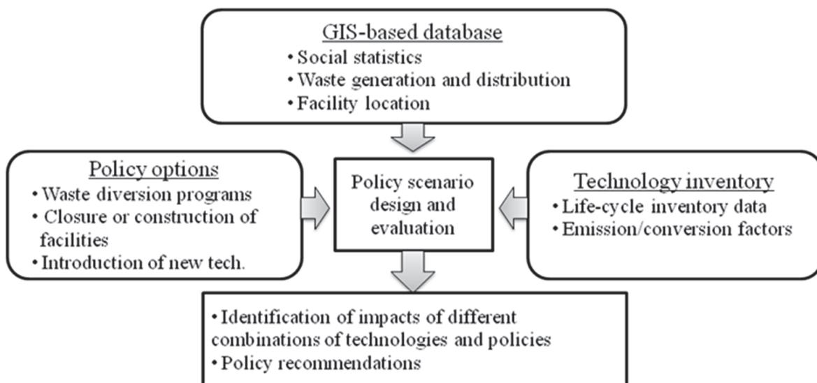
Fig. 1. Urban environmental technology simulation system for recycling
