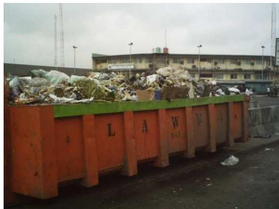
Fig. 5. External bins for storing solid waste before collection by disposal agents
