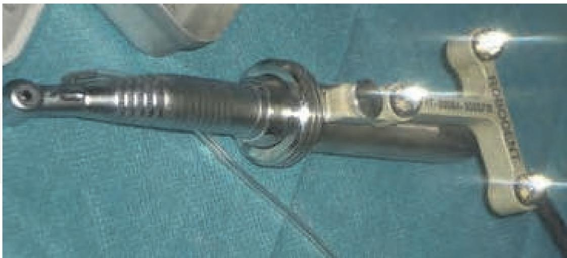
Fig. 20. a and b: Robodent: radiological guide and the extremity of drill present optical marks to give the spatial position.
