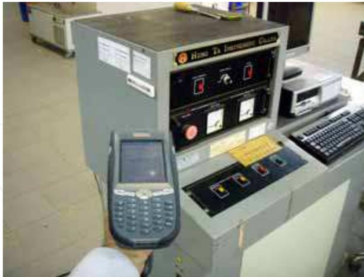
Fig. 6. Displayed maintenance staff member used RFID-enabled PDA to scan RFID tags (2).
