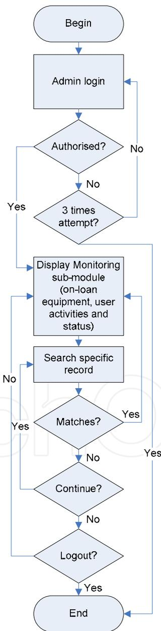
Fig. 10. The system flow of data monitoring module
