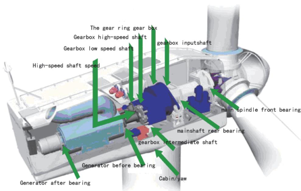
Fig. 11. The scheme of fans' monitoring
