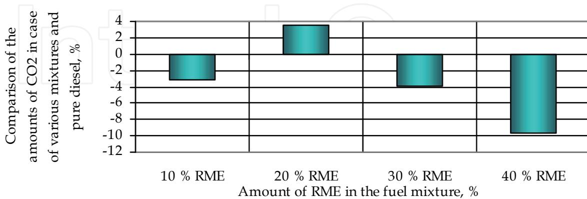
Fig. 18. Comparison of CO<sub>2</sub> emission in case of various mixtures to emission when using pure diesel
