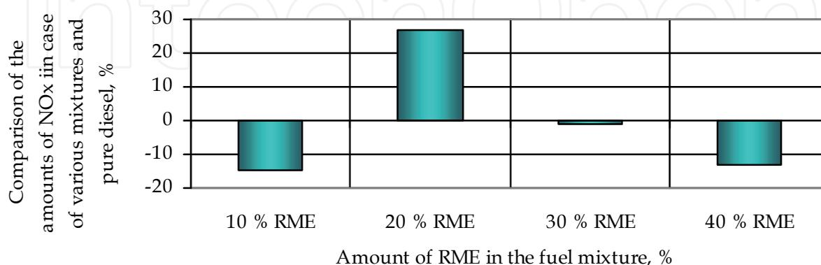
Fig. 17. Comparison of NO<sub>x</sub> emission in case of various mixtures to emission when using pure diesel
