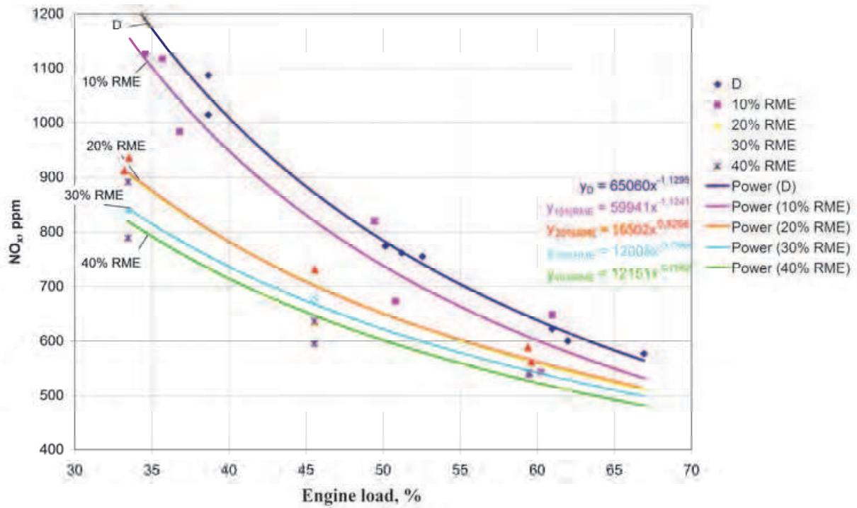
Fig. 10. Dependence of emission of nitrogen oxides on the engine power (% P<sub>max</sub>) when using various fuel mixtures
