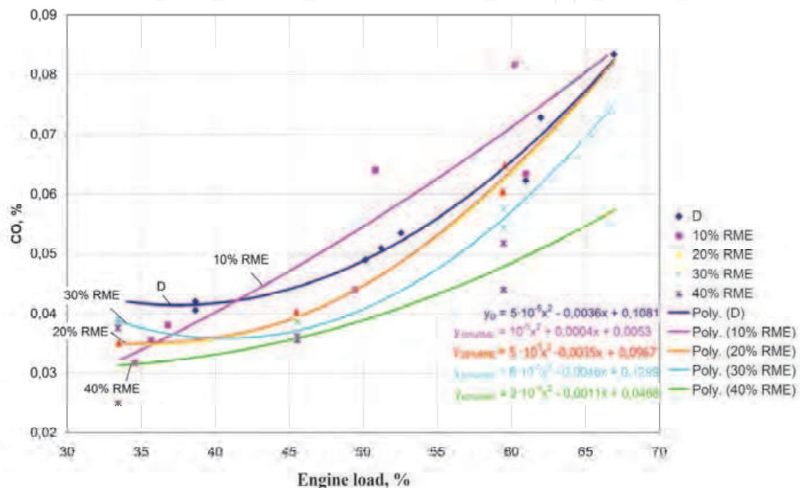
Fig. 12. Dependence of emission of CO on the engine power (% P<sub>max</sub>) when using various fuel mixtures
