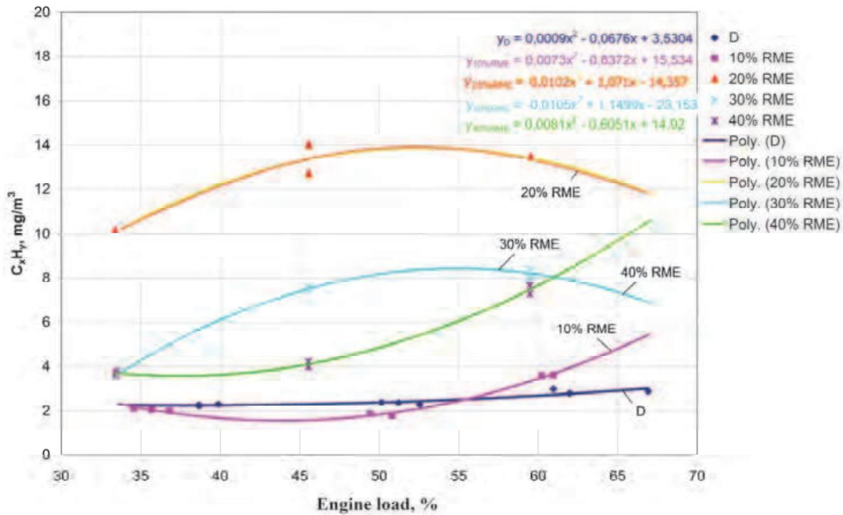
Fig. 14. Dependence of emission of CxHy on the engine power (% P<sub>max</sub>) when using various fuel mixtures
