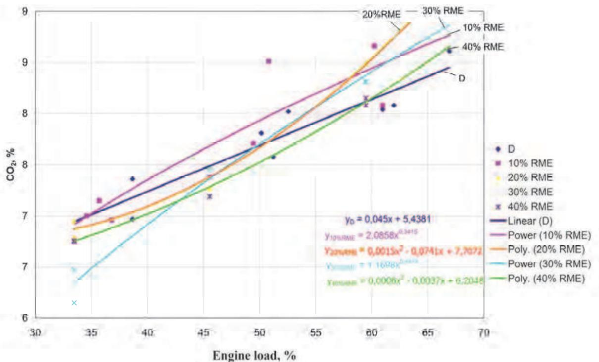
Fig. 11. Dependence of emission of CO<sub>2</sub> on the engine power (% P<sub>max</sub>) when using various fuel mixtures
