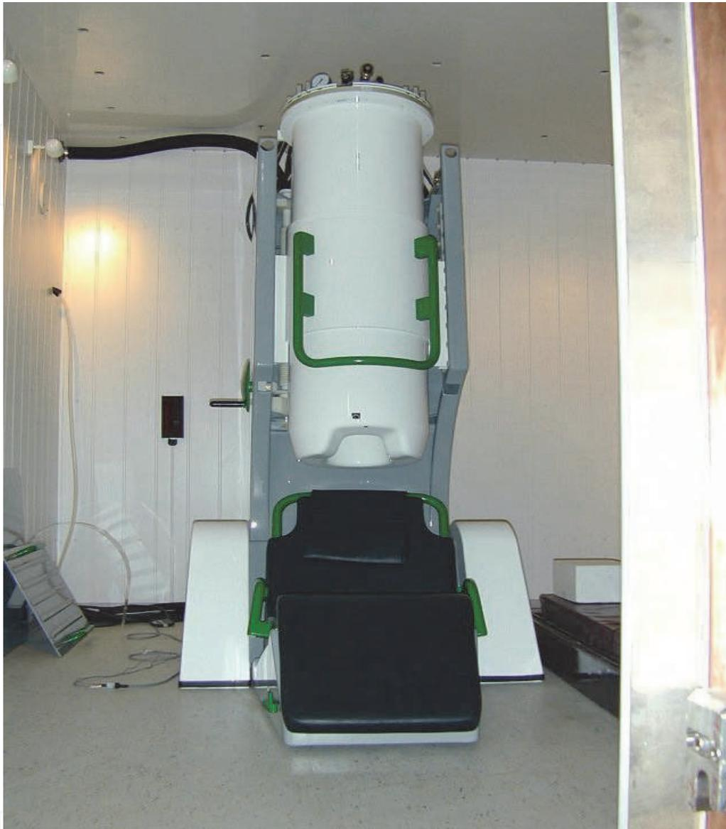
Fig. 1. The 122-channel-biomagnetometer
