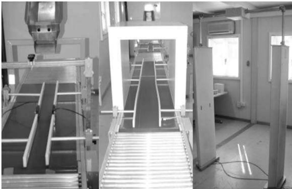
Fig. 3. Test environment to simulate the supply chain
