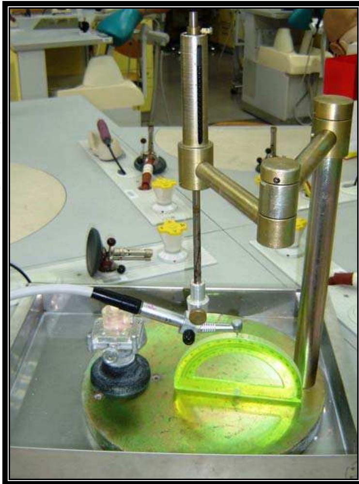
Fig. 2. The paralleling apparatus used
