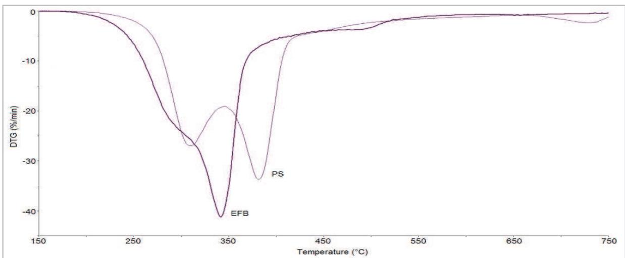
Fig. 5. EFB and PS DTG curves at 50 °C/min
