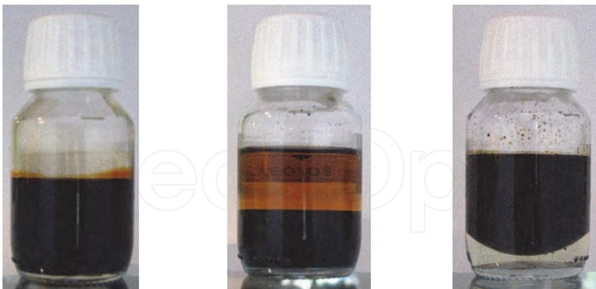
Fig. 5. Pictures of pyrolysis oil (left), mild HDO (middle) and 2<sup>nd</sup> stage HDO (right) products
