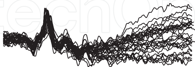
Fig. 3. Fifteen serial ERG recordings from 15 Espion e 2 (Diagnosys LLC, Lowell, MA) electrodiagnostic instruments. ERGs were recorded to 3 cd s/m 2 flash through undilated pupils in a single subject, ND using DTL-Plus Diagnosys LLC, Lowell, MA) microconductive fiber electrode. A: ERGs were repeated at each site to demonstrate replicability. B: Overlay of all recordings demonstrates consistent A and B wave response amplitudes and latencies across all recordings. ( The authors would like to thank Natalie Doran and Diagnosys LLC for providing the ERGs used in this illustration. )
