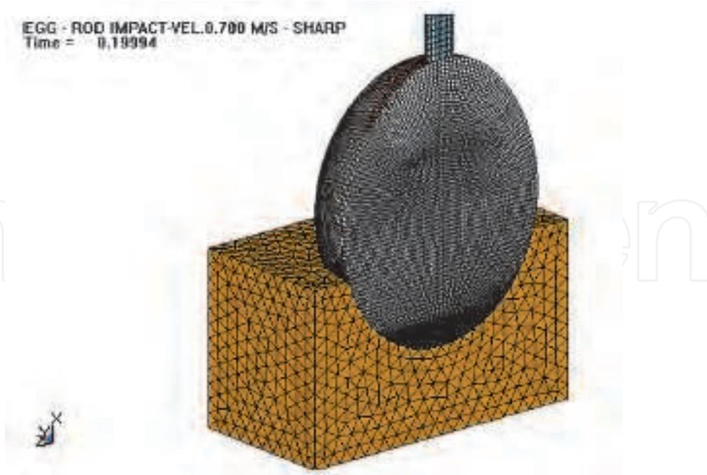
Fig. 9. Numerical model of the experimental set-up.
