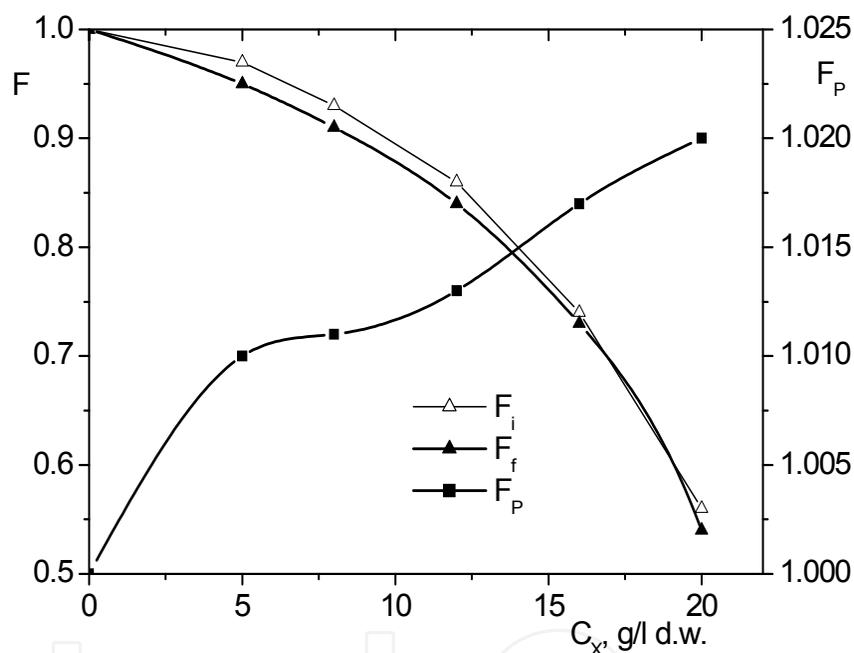
Fig. 5. Influence of biomass concentration,  $C_X$ , on factors  $F$  and  $F_P$  for facilitated pertraction from *S. erythreus* broths (pH of feed phase = 4, pH of stripping phase = 2, carrier concentration = 40 g/l, rotation speed = 500 rpm)
