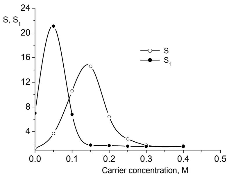
Fig. 12. Influence of carrier concentration on selectivity factors (citric acid concentration in feed phase =  $7.8 \times 10^{-2}$  M, malic acid concentration in feed phase =  $7.8 \times 10^{-2}$  M, succinic acid concentration in feed phase =  $7.8 \times 10^{-2}$  M, rotation speed = 500 rpm)
