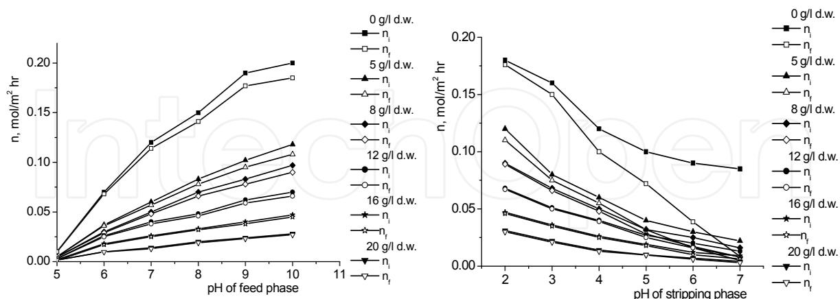
Fig. 3. Influence of pH-values of feed and stripping phases on initial,  $n_i$ , and final,  $n_f$ , mass flows of Erythromycin for free pertraction from *S. erythreus* broths (rotation speed = 500 rpm)
