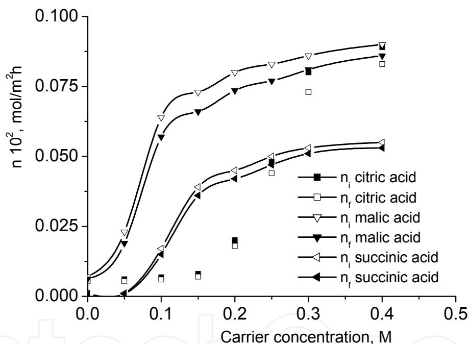
Fig. 11. Influence of carrier concentration on citric, malic and succinic acids mass flows (citric acid concentration in feed phase =  $7.8 \times 10^{-2}$  M, malic acid concentration in feed phase =  $7.8 \times 10^{-2}$  M, succinic acid concentration in feed phase =  $7.8 \times 10^{-2}$  M, rotation speed = 500 rpm, pH of feed phase = 3, pH of stripping phase = 11)
