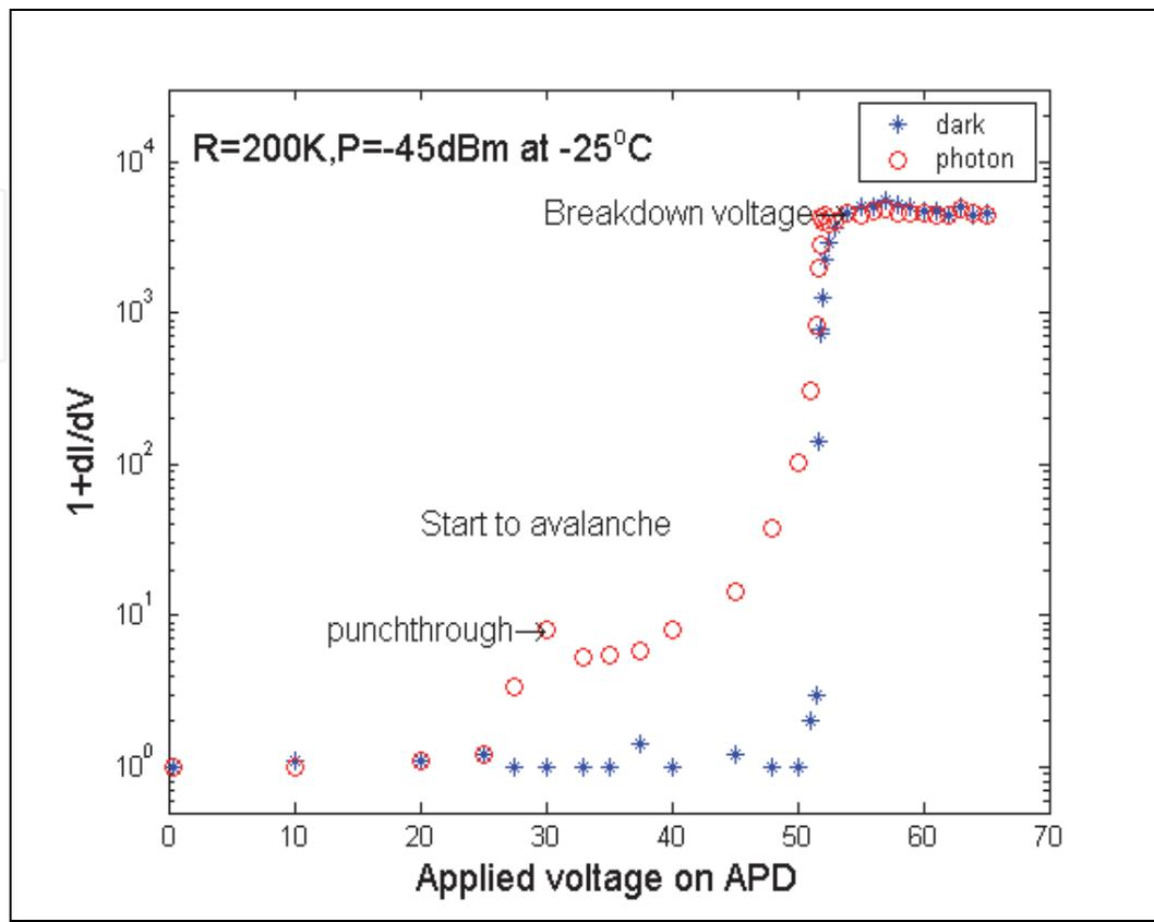
Fig. 8. The relative current gain versus bias characterization curves clearly indicating the punch through voltage, breakdown voltage and the avalanche.
