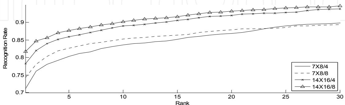
Fig. 4. Comparison of recognition rate for different blocking number and sampling density for RIU-LBP (With sampling radius 2, image resolution  $70 \times 80$  and  $7 \times 8 / 4$  denotes blocking number  $7 \times 8$  and sampling density 4)
