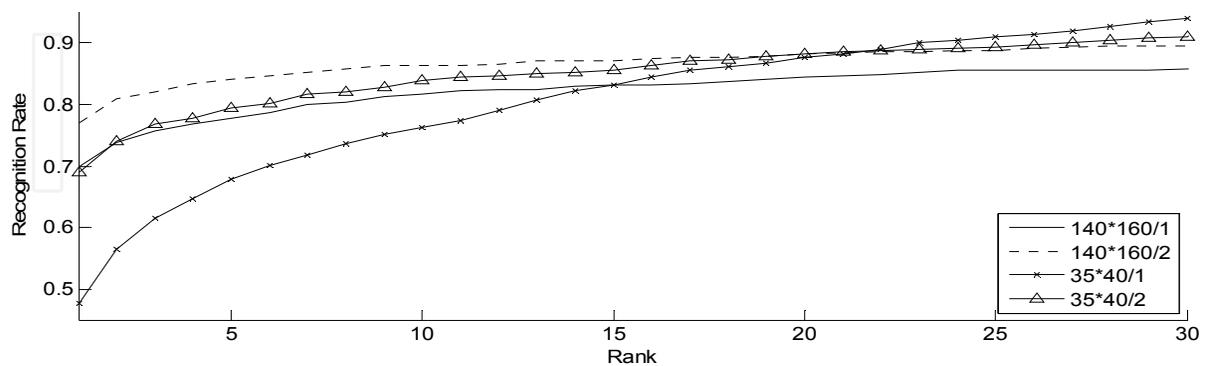
Fig. 5. Comparison of recognition rate for different sampling radius and image resolution for RIU-LBP (With blocking number  $7 \times 8$ , sampling density 8 and  $140 \times 160/1$  denotes image resolution  $140 \times 160$  and sampling radius 1)
