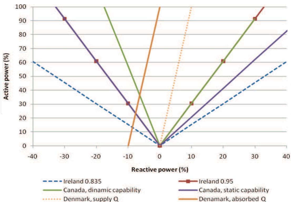
Fig. 2. Reactive power requirement for several grid codes.
