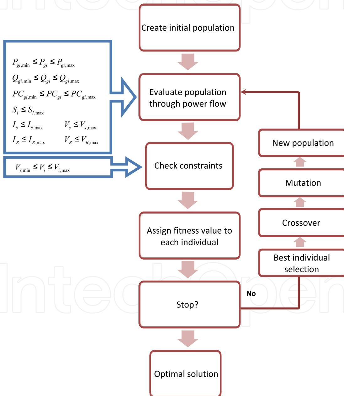
Fig. 5. Flowchart of optimization process
